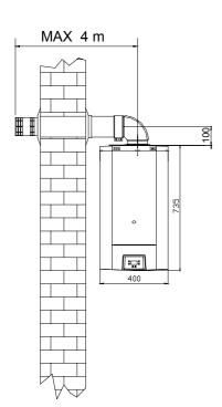
N.B.: The allowed lenght of coaxial flue ducts is by a minimum 0,5 meters to a maximum of 4 meters.
