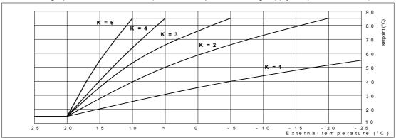
The regulation of the ambient temperature can be made only by compensation of supply temperature with the external temperature or in combination with the remote control (look at instruction manual of remote control).
