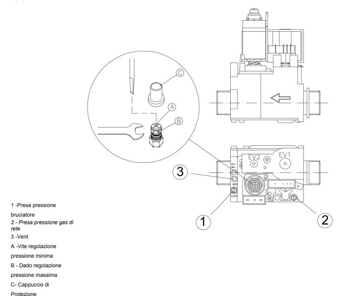
To perform the control of the pressures to the burner, to insert the probes of the manometer in the available takings of pressure on the valve gas (you see fig.).
