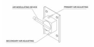
The combustion air flows through the suction port and duct located behind the combustion air modulating device. The air entering the boiler is then divided in two separate streams called "primary combustion air" and "secondary combustion air".
