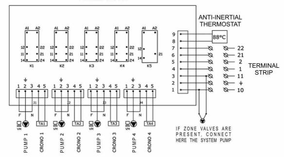
WARNING: THE MAXIMUM CURRENT MUST BE LESS THAN 4 AMPS
