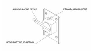
The combustion air flows through the suction port and duct located behind the combustion air modulating device. The air entering the boiler is then divided in two separate streams called "primary combustion air" and "secondary combustion air".
