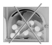
**NOTE**: This instructions must be strictly followed. Since it is necessary that the wood come down smoothly and evenly in the fuel chamber in order to have good combustion, make sure that the wood logs' dimensions, shapes and the loading pattern don't create obstacles to movement. The wood logs must be loaded longitudinally, no piece must be put in a raking way or transversely.
