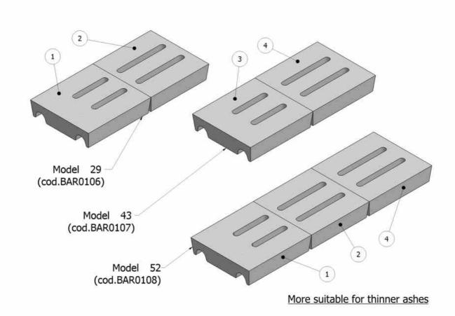
**Mounting warnings:** the piece with longer slots must first be firstly positioned on the boiler back plate side. The grate with longitudinal slots (pic. 1,2,3,4) is better suited to types of wood producing thinner ashes. When the grate is changed, the authorized technical personnel must consider employing the best suitable new type.
